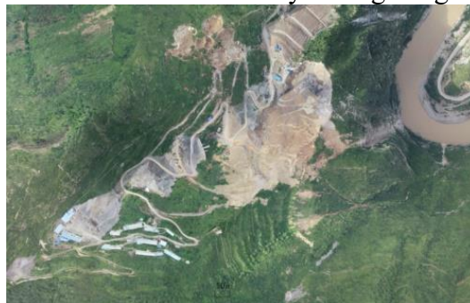
Figure 4: This is a orthophoto image created from UAV aerial images. On the map, we can see the scope of the construction impact, and can speculate on the area where the disaster may occur. In addition, the final affected area can be judged according to the gully and the range of water flow after the river is relocated.
