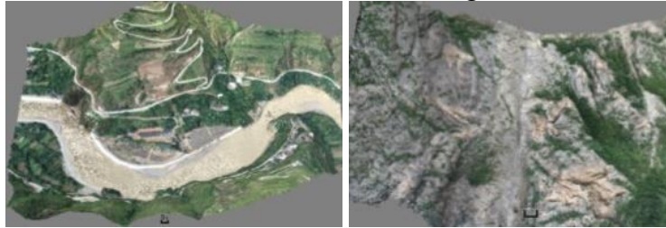
Figure 1: Region scale model and outcrop scale model. In order to fully express the shape of the geological body through the model during UAV aerial photography, we should select the appropriate shooting angle to ensure that the geological information from all angles of the object can be fully expressed. For areas with relatively small topographic relief, the main shooting mode is direct flight, and detailed geological information can be ensured through UAV camera angle.
